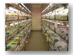
An operator of an in-vitro production facility has several possibilities to minimize the energy costs. One of these is the choice to illuminate the plants with light at night, when the tariff of electricity is reasonable low. Another possibility is installing energy-saving light sources, which can bring a small improvement, but much better savings come from making the use of the new developed light technique.
